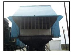
Work on this item has been deferred in anticipation of returning the trailer to the factory. The trailer structure does not provide a support system for moving the gas generator forward for access; therefore this work is better suited for the factory.
